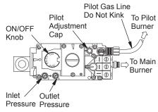
Figure 13 - Millivolt Control Valve
